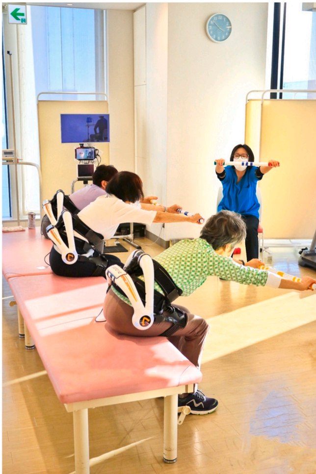
Fig. 3. Trunk forward/backward tilt training with the Hybrid Assistive Limb lumbar type.
